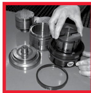
Re-install the original punch driver supplied with the guide to convert the guide for use with conventional Strippit style tooling.
