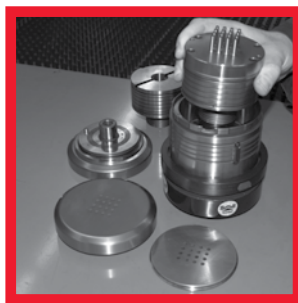
Use the quick release features on the guide assembly to disassemble the cluster. Unscrew the integral punch driver assembly.
