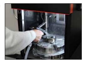
The Coolant Sprayer allows the part to be rinsed prior to its removal from the machine, and easy cleaning of the fixture and work area.
