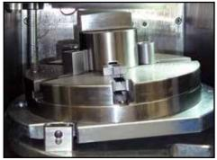
**The Premia Sharpening System includes** a graduated angle plate that allows a shear (rooftop, whisper, or one-way) to be ground on to punches easily. Simply tilt the plate and use the graduated cam to select the appropriate angle up to 12°.
