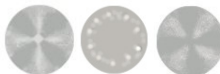
Figure 3b. Uneven coloration indicates mechanical or thermal stress and potential failure. Lens replacement is recommended.
