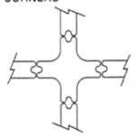
4-Way Radius tool (center) with micro-joint ends, paired with slitting tool, to create "shake-and-break" application.
